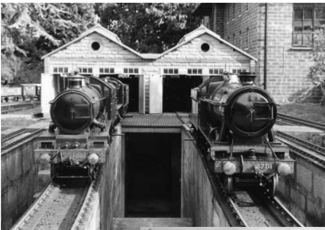
GWR super-power on the 7.25" gauge at Thame, where 4-6-0 4082 'Windsor Castle' and 2-8-0 4701 stand over the pit outside the loco shed.
