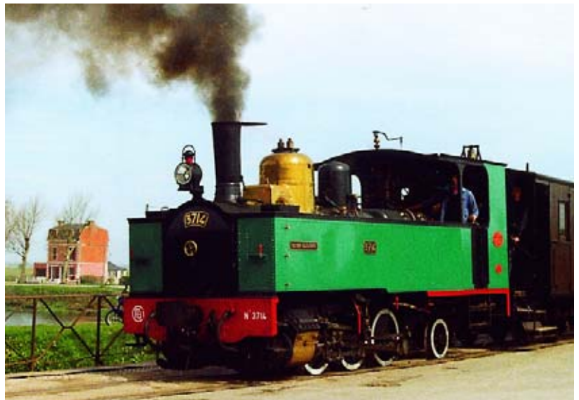
Built by Buffaud & Robatel in 1909 0-6-2 No. 3714 Beton Bazoches with open fronted cab through several hands before restoration by the CFBS 1972 - 81. Eddie Lewcock April 2000
