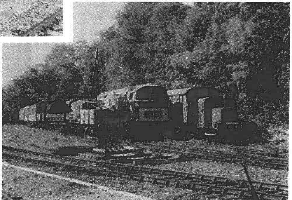
ABOVE: Like many embryonic steam railways the Bodmin & Wadebridge relies on industrials for its motive power. Typical is No.19 a Bagnall 0-4-OST previously employed by HM Dockyard Devonport and seen running round at Bodmin Parkway.
