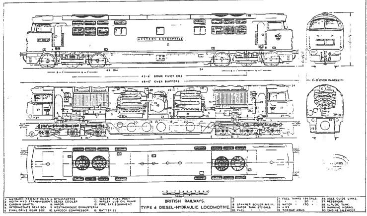
stator back to the impeliar, the oil being constantly circulated whilst the locomotive is in motion. The diesel-hydraulics gearboxes are fixed ratio units which distribute and redirect the drive.
