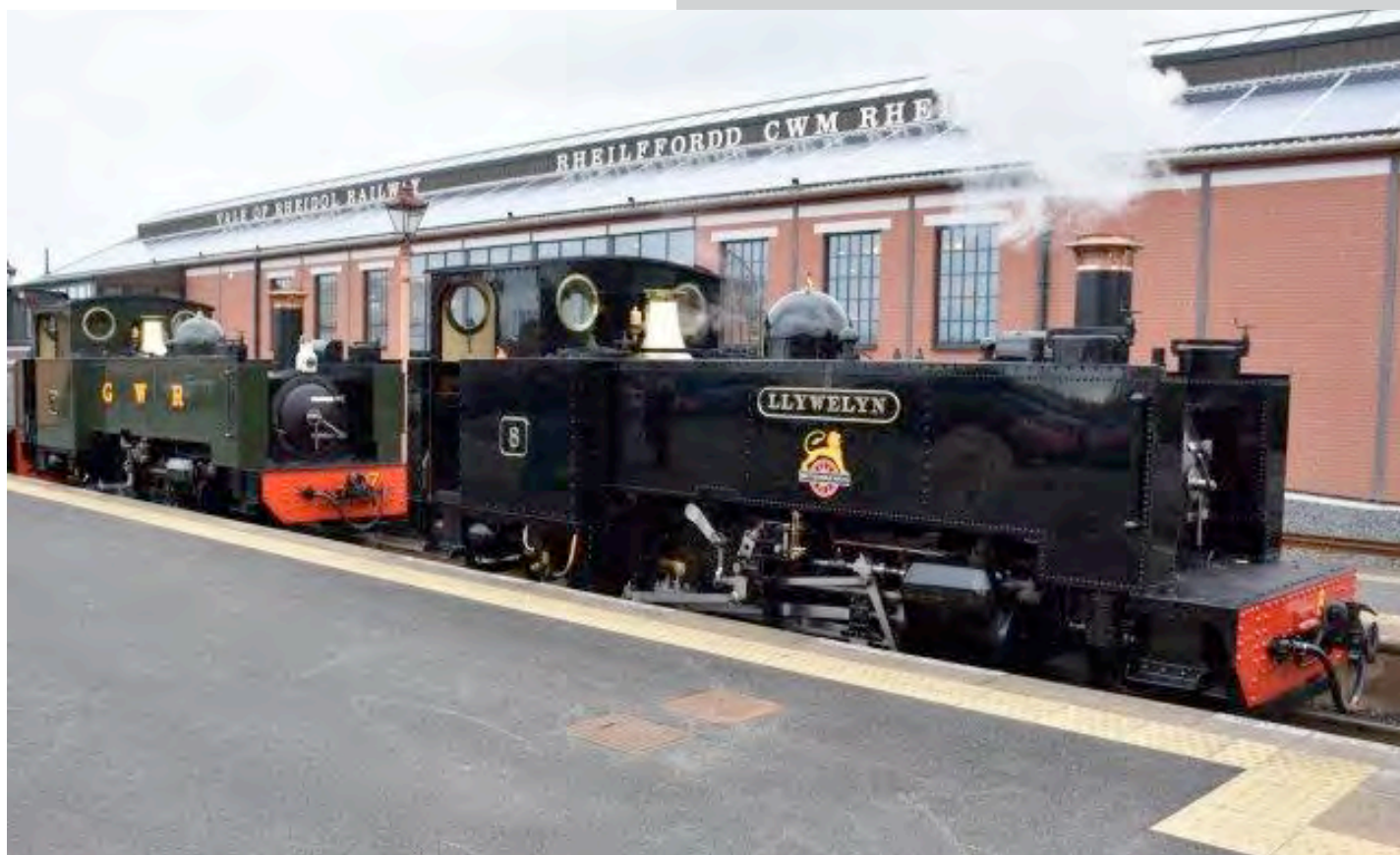
GWR 2-6-2 Rheidol Tanks – No.7 in unlined GWR Green livery and No.8 in unlined BR Black with early 'Lion over Wheel' emblem and 'Llywelyn' nameplate.
