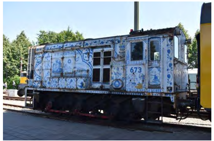
0-6-0 Shunter 673 built Dick Kerr Works, Preston 1955-6. Originally 605 it was renumbered when a radio transmitter was fitted to allow remote control in the 1990s. The livery is reminiscent of Delft pottery.
