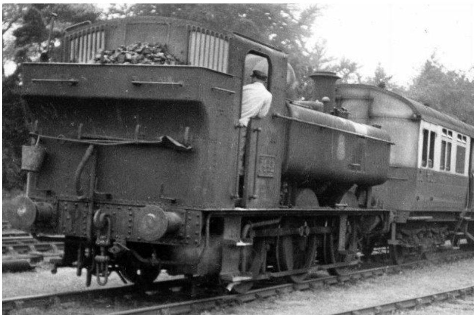
7442 at Watlington on 23rd June 1951 showing the square joint between cab and bunker also found on the later 64XX locos. R. S. Carpenter
