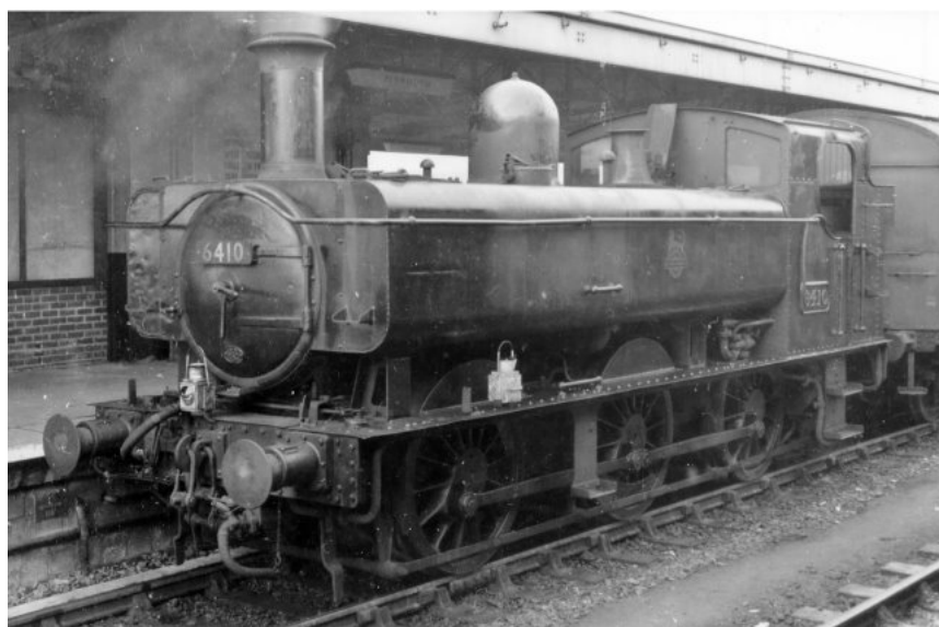
6410 at Plymouth North Road in 1959/60 in plain black with the early emblem. The smaller splashers identify this class whilst the 54XX, 64XX and 74XX classes all have drumhead smokeboxes and the tanks covering the boiler tops.
