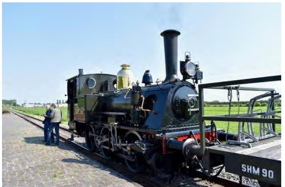
Stoomtram's former NS loco No 7742 Bello an 0-6-0 WT Built by L. Schwartzkopff of Berlin in 1914 stands at Wognum whilst passengers take a look at the station, shop and small museum on 8th June 2023.
