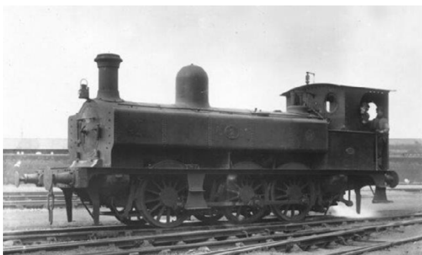
Cardiff Railway no.2, later GWR 693 a Kitson "Long Boiler" 0-6-0 built as a pannier tank in original condition.
