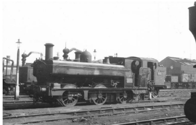
2120 in late condition with enclosed cab. Both the 850 and 2021 classes can be spotted by the buffer beams protruding above the running plate. The 2021s had conventional spokes.
