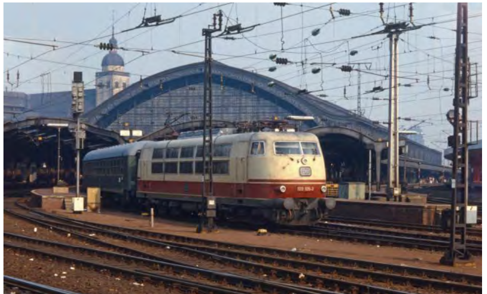
Another DB modern classic: 7,780kw Co-Co No.103.105 (Krauss Maffei 19465/1970) departing from Köln Hbf on 10th June 1979
