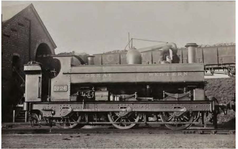
1026, one of the first batch of the 1016 class, at Reading shed on 18th October 1919 shortly after being fitted with Q class boiler and small pannier tanks. Later, the tanks were slightly deeper.
