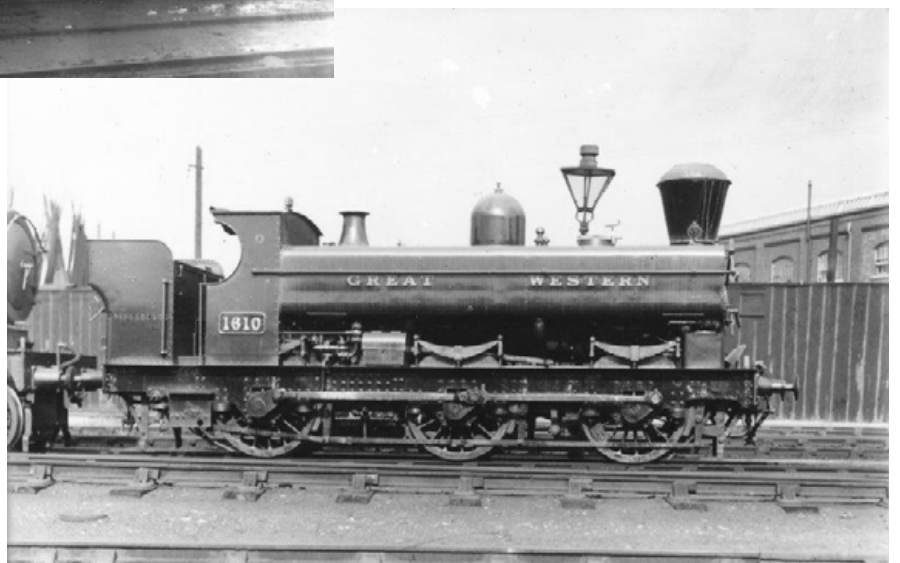
Another 1076 class 1610 built as a standard gauge saddle tank but seen at Swindon on 11th September 1927 fitted with pannier tanks and a spark arrestor but retaining its open cab.
