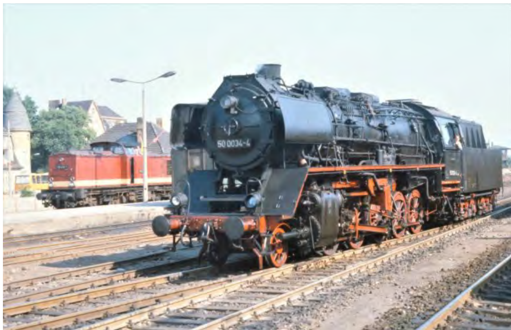
DR 2-10-0 No.50.0034 (BMAG 11858/1942), one of the legendary Kriegsloks, and 736kw B-B diesel hydraulic No.110.416 (LEW 12925/1971) at Angermünde on 5th June 1979.
