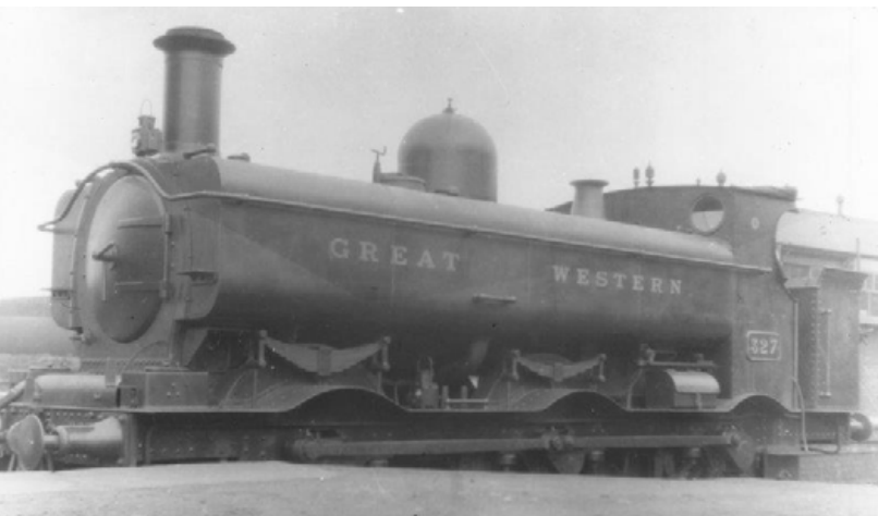
322 class no.327 which started life as a 0-6-0 tender locomotive and seen here late in its life with a P class boiler and pannier tanks.
