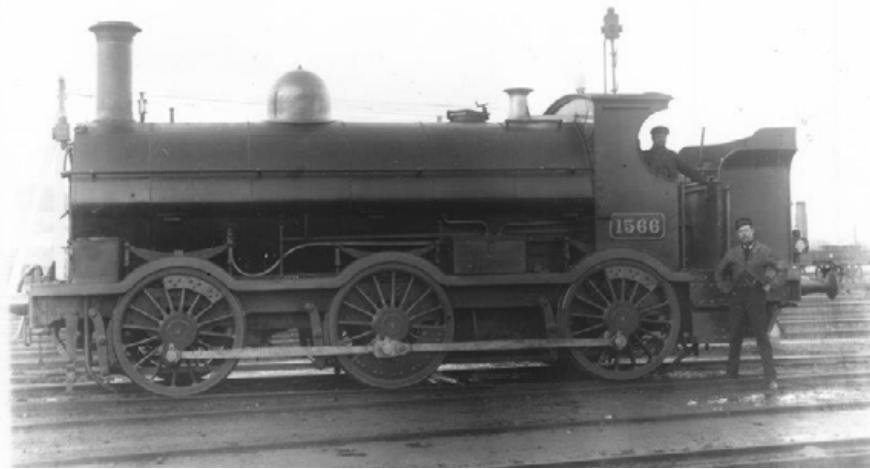
1076 class convertible 1566 in broad gauge guise circa 1884-92. Note the wheels are outside the frames.
