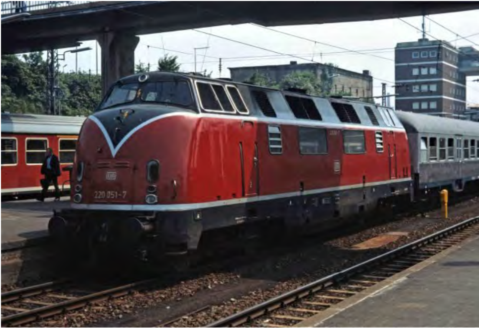
DB 2,200hp B-B diesel hydraulic 220.051 (Krauss Maffei 18295/1957) at Osnabrück Hbf on 2nd June 1979.
