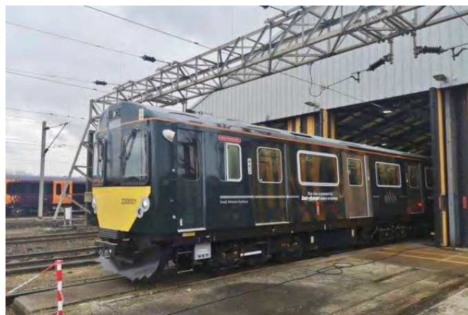
The prototype Vivarail Class 230 unit was converted to battery electric operation and has now been acquired by GWR whose livery it now carries. It is seen at Bletchley depot.
