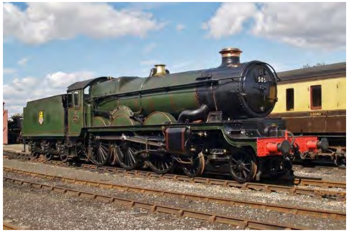
5051 Earl Bathurst , also at Didcot, has the later pattern valve chest cover which was later fitted to most of the earlier locomotives and the short cover on the smokebox side associated with the 3-row superheater. It is also coupled to one of the Hawksworth-pattern flush sided 4,000 gallon welded tenders introduced in 1946.
