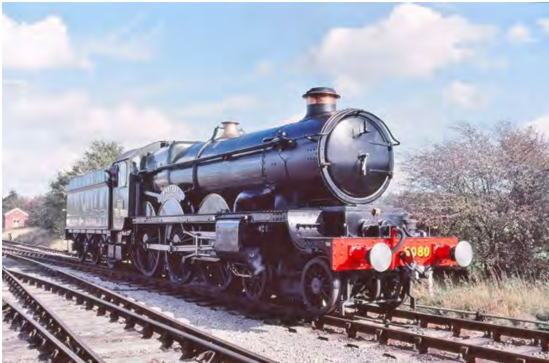
5080 Defiant at Toddington on 14th October 1990 during a visit to the Gloucestershire - Warwickshire Railway. The locomotive retains its original single chimney and 3-row superheater.
