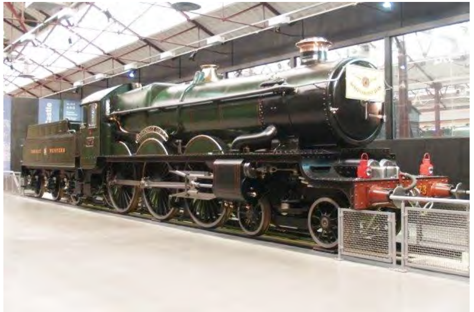
The pioneer Castle, 4073 Caerphilly Castle on display at Steam in Swindon fully restored to original condition including the low-sided 3,500 gallon tender.
