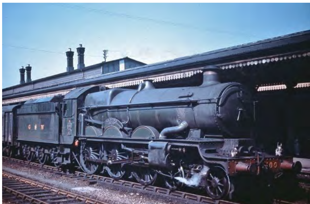
A rare view of 100 A1 Lloyds on an Up train at Reading in April 1947 during the brief period it was running as an oil-burner; note the tank in the tender coal space.
