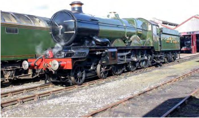
4079 Pendennis Castle as now restored at Didcot exhibits the original concave casing around the inside cylinder valve chests fitted to 4073-4099/5000-5012. It is also coupled to the standard Collett-pattern 4,000 gallon tender with flared sides.
