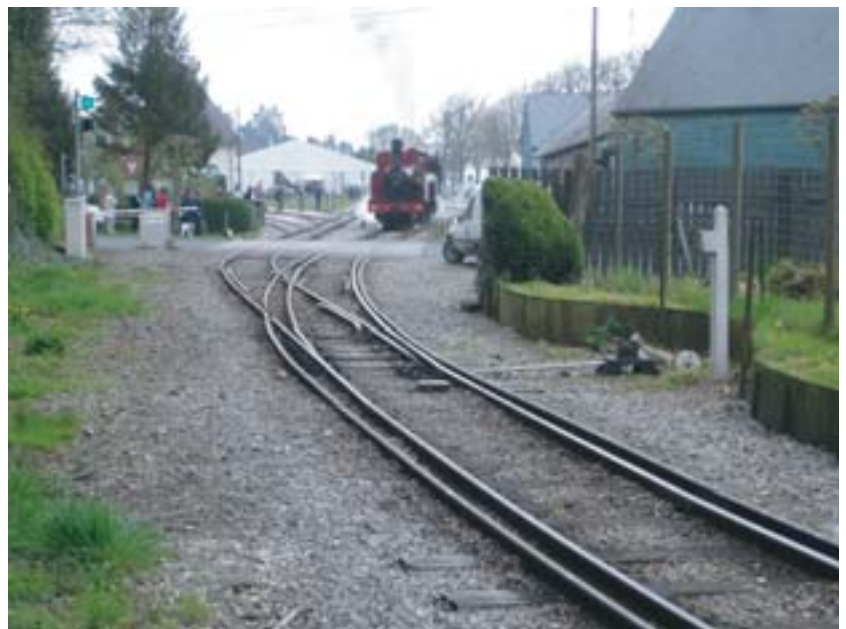
These two photographs show the complications of mixed standard and metre gauge tracks on the C F Baie de Somme. Note that here there are separate rails for each gauge.
