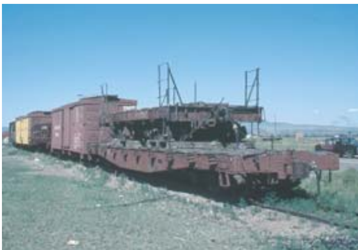
One of the DRGW coupling converter cars (stabled on top of a standard gauge flat car) note the narrow gauge coupler pocket below and left of the standard gauge one.
