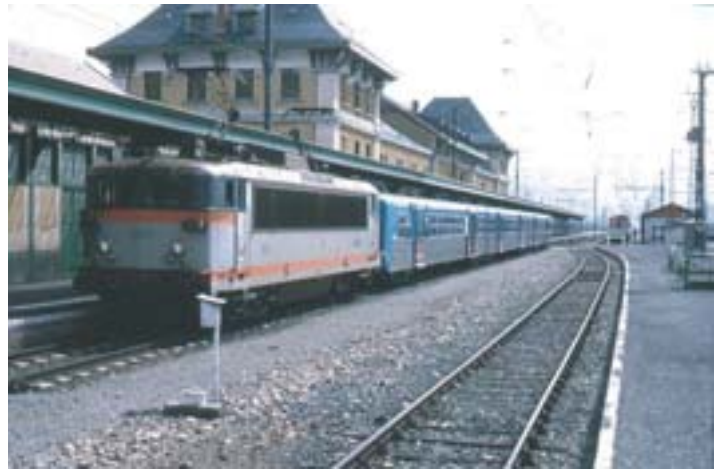
At La Tour-de-Carolain on the French-Spanish border three gauges share the same station. Left: A 5' 6" gauge EMU of the Spanish State Railways (RENFE) stands alongside the standard gauge tracks of the French SNCF. On the left is a metre gauge EMU of the Petit Train Jaune de le Cerdagne (Little Yellow Train) that makes a spectacular 63km journey through the the mountains from Villefrance de Conflent via France's highest station at 1593m. it is electrified at 850VDC with a slightly raised 3rd rail. Right: SNCF 8833 stands at the left hand platform with the RENFE train visible in the background. two photos: Tim Speechley
