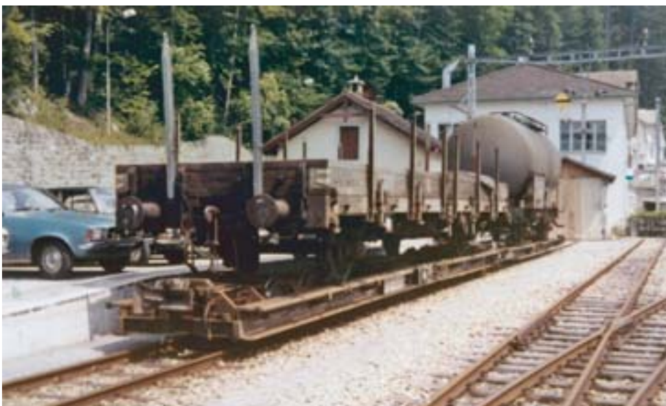
Standard gauge wagons being carried piggy-back style on metre gauge transporter wagons on the Swiss Federal's Lucerne to Interlaken line at Brienz. photo: Mike Walker
