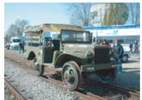
Amongst the oddities operating at Noyelles was this ex-US Army WWII Dodge truck converted for standard gauge use.
