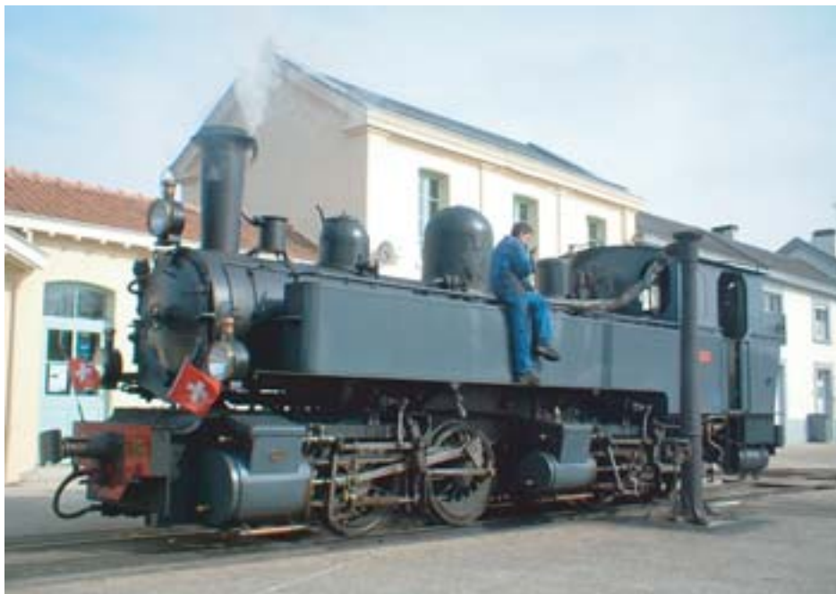
Ex Portuguese Railways E194, a German built 0-4+4-0T, takes water at Noyelles on the Friday afternoon whilst working a test train. This loco had been brought 850 km by low loader from Switzerland to participate.
