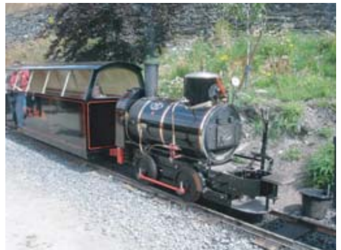
Ant of the Laxey Mines Railway. Note the primitive driving position. The "dome" is actually the water tank!
