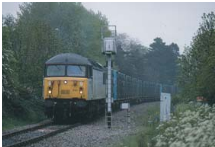
On the former LNWR route to Oxford, 56041 approaches the level crossing at Bicester Town with a train of 'binliner' empties from Calvert on 17 May 1991. The train was held at this signal whilst a Bicester Town to Oxford DMU cleared the block to Oxford North Jct.
