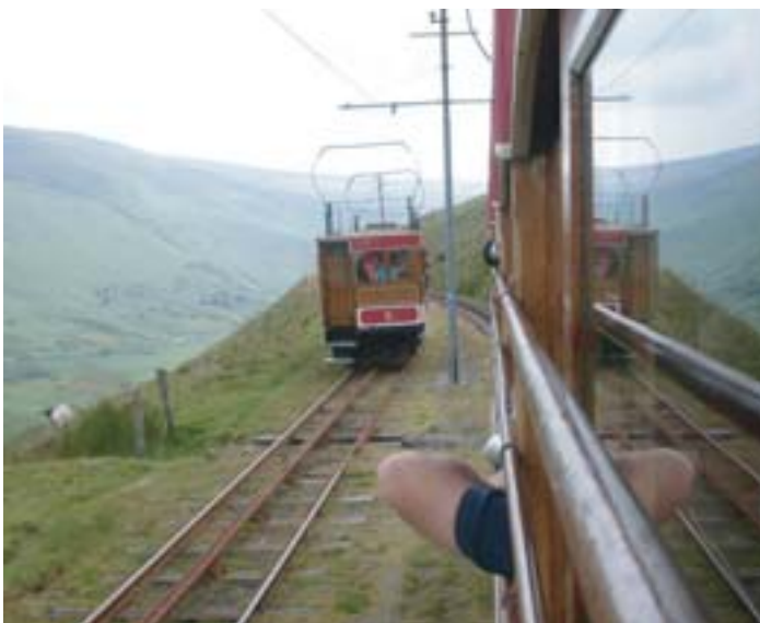
Snaefell Mountain cars pass under the watchful eye of a local sheep. The horizontal rail gripped by the Fell emergency brakes can be seen between the running lines.
