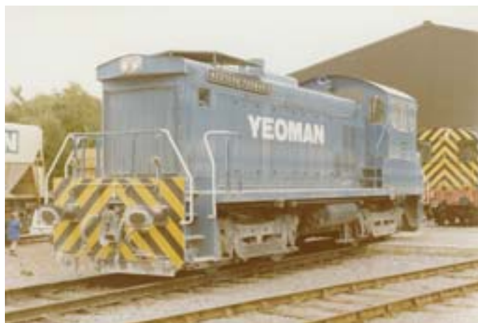
First contact. In early 1981 Foster Yeoman took delivery of the first GM built loco to operate on the British mainland, An almost standard model SW1001 "switcher", no.44 Western Yeoman II is seen at Merehead during its first year of service.
