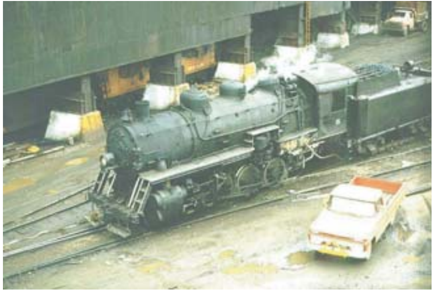
Northwest Steel & Wire 15 in front of the electric furnace building at the Sterling, Illinois, mill in September 1965. The 0-8-0 was built by ALCo in 1923 for the Grand Trunk Western as its 8315 and later got a tender from a Chicago Burlington & Quincy 2-8-2.
