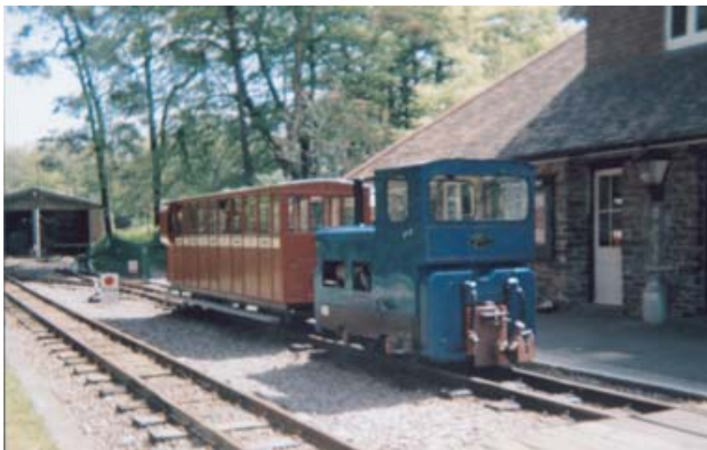
For the present, internal combustion power is the order of the day for the fledgling Lynton & Barnstaple Railway. An 0-4-0 Simplex was the motive power on 11th May 2005 and is seen in the sylvan surroundings of Woody Bay station.
