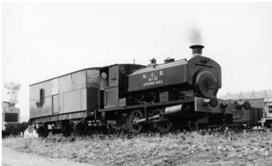
In pouring rain, former NCB Waterside 0-4-0ST No.10 (Andrew Barclay 2244/1947) gets up steam ready for the inaugural rides at the Scottish Industrial Railway Museum on 24 June 1990.
