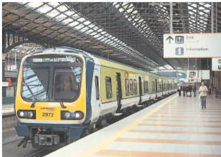
The new order. One of twenty 4-car diesel-hydraulic multiple units recently delivered to Irish Rail by CAF from Spain for working the outer suburban services around Dublin stands at Dublin Connolly on a Drogheda service on 9 May 2004.
