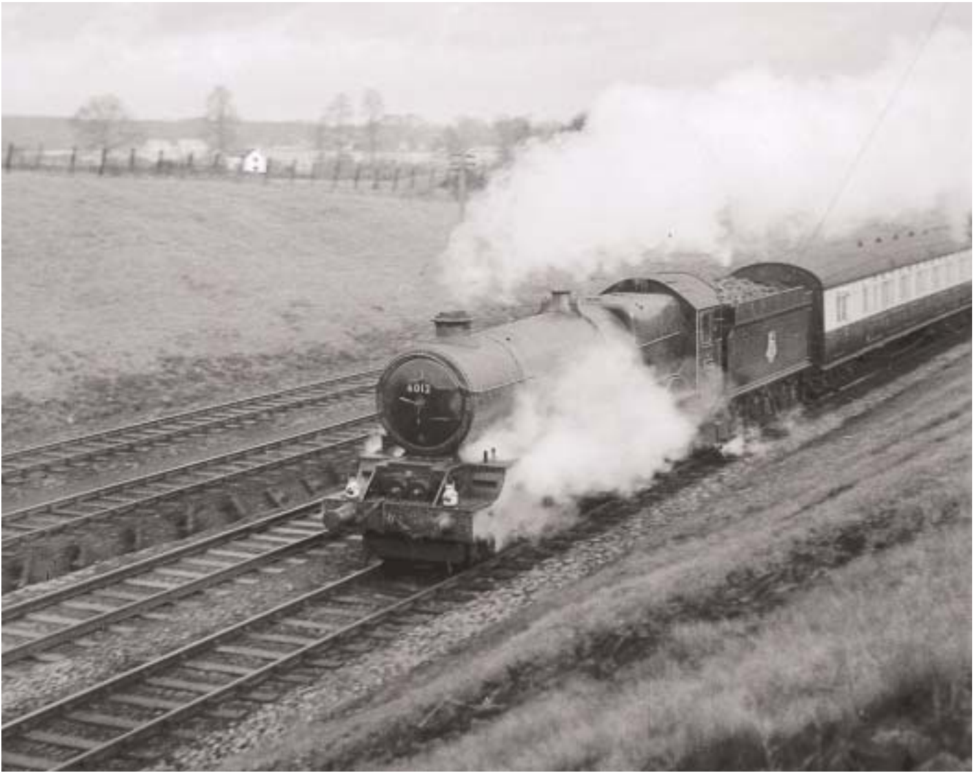
6012 King Edward VI on the down main Maidenhead nr. West Box. Built April 1928. Double chimney fitted February 1958. Withdrawn September 1962. Early 1950s - Ken Laurie
