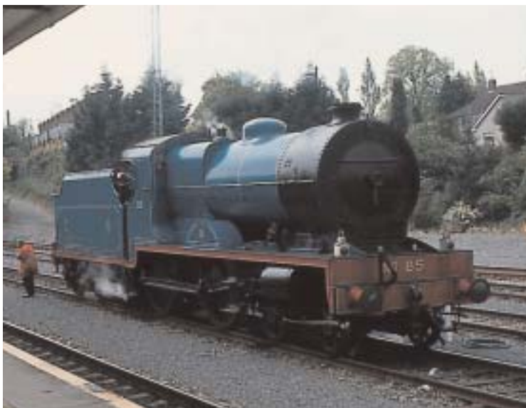
Former Great Northern Railway (Ireland) 85 Merlin, a V class 4-4-0 three cylinder compound built by Beyer Peacock in 1932, waits at Dundalk prior to heading the RPSI Slieve Kinalta tour onward to Belfast and Bangor on 10 May 2004
