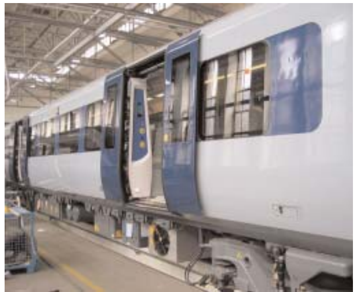
Below: Those suburban doors - note the beam for the collector shoe. Final livery. First class will have the cant rail stripe
