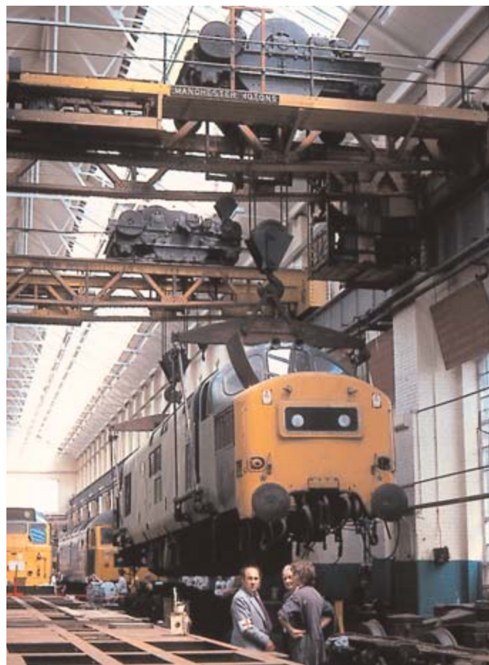
Inside the Traction Repair Shed, 37 160 is lifted off its bogies by the overhead crane at the Stratford Open Day, 14 July 1979.
