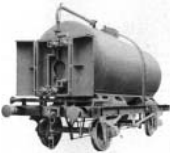
4-wheel Oil Tank Wagon, "TO" Type, for Pakistan Railways, 3' 6" gauge.
