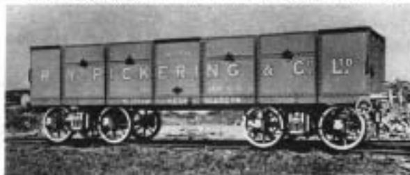
25-ton Bogie Wagon (one of the earliest built in Scotland)
