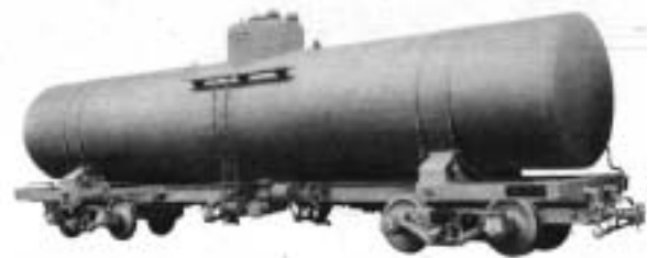
Bogie Oil Tank Wagon for East African Railways (Kenya Section), Metro gauge.
