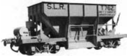
Bogie Side Discharge Hopper Wagon for Sierra Leone Railway, 2' 6" gauge.
