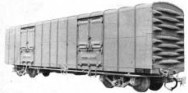
Bogie Covered Goods Wagon for East African Railways (Tanganyika Section), Metro gauge.
