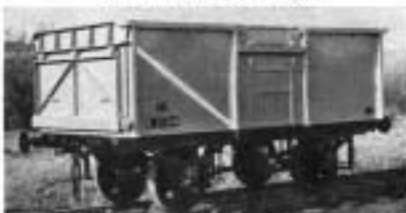
16-ton Steel Coal Wagon
